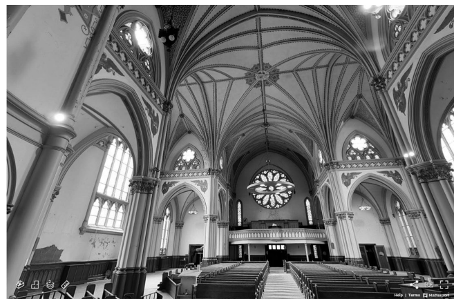
Figure 3. Matterport screen capture of St. Mary’s. The photogrammetric scan is accessible in a virtual viewer, enabling students to understand color, material, finish, take measurements, and make interactive walk-throughs of any room. Virtual model by Owen Bush & Scan2Plan, 2021.
